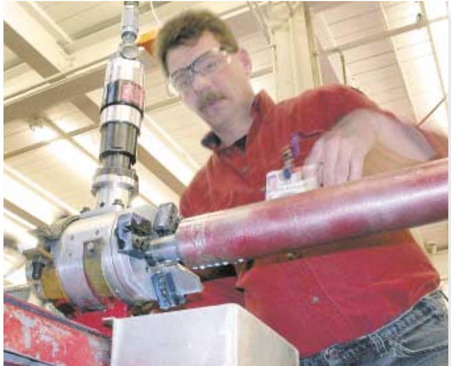
*Pipefitter Alan Duperry (243) uses end-prep equipment in the Wet Dock Pipe Shop to cut a 45-degree bevel on a section of pipe.*
