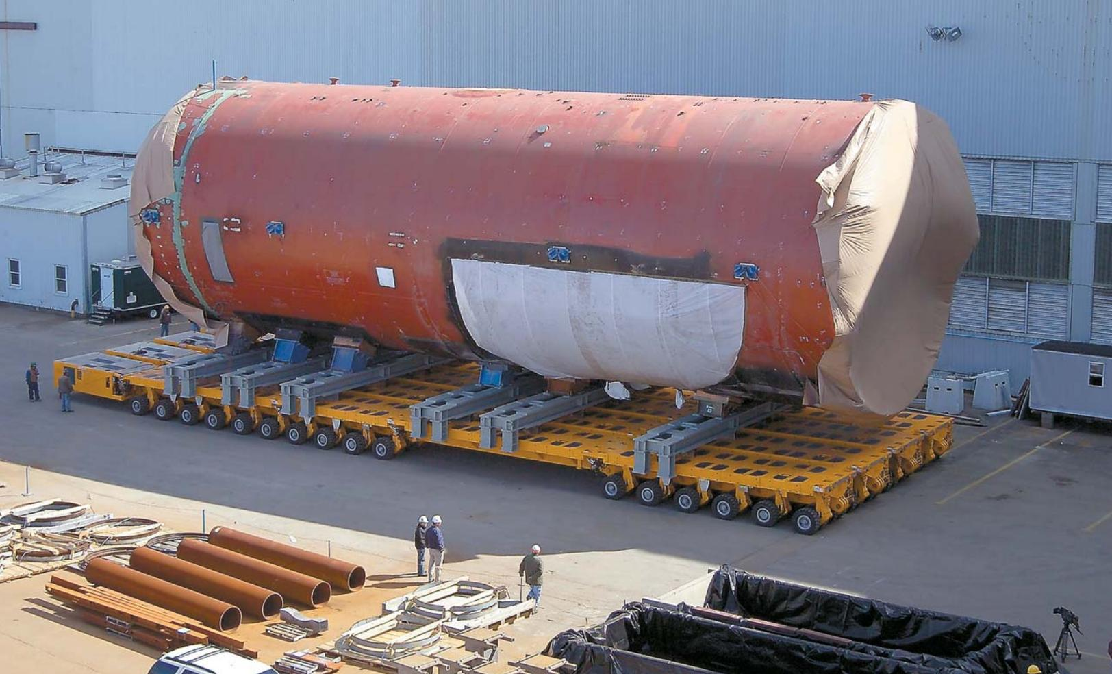
Using the new heavy-lift system, Section 2B-5 of the North Carolina moves into Quonset Point's new Coating Facility. The move was the first for the new heavy-lift system and it's the first unit to enter the new building.
