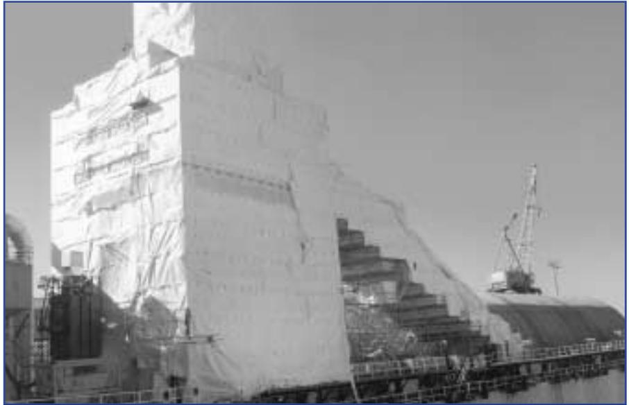
The center wall Clyde, shrouded for blast and paint operations, is undergoing major renovations in anticipation of additional work from the Navy submarine base.
