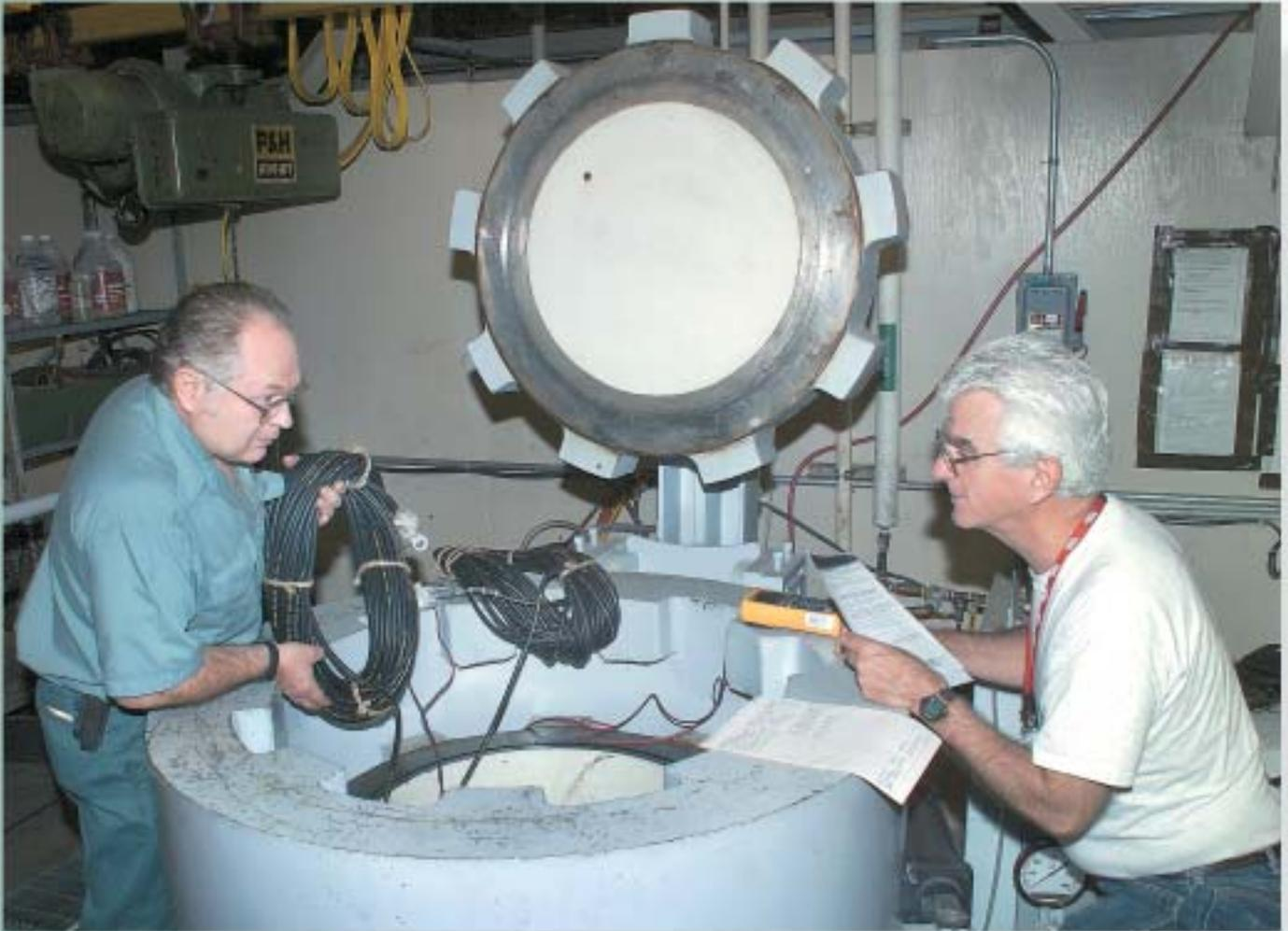
From left, vulcanizing technicians Gerry Tanguay and Ed Frink (both of 241) prepare to load cables into Electric Boat's new pressure tank, which has made the process of conducting hydrostatic tests on external submarine cables much less physically demanding.
